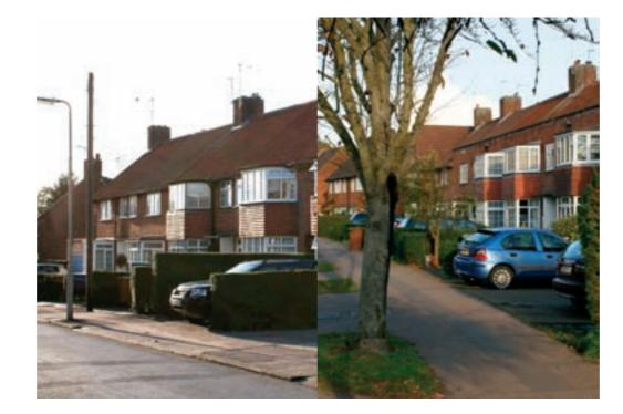
The space for a single hard standing for a car must be no less than  $4.8 \times 2.4 \text{m}$ .
